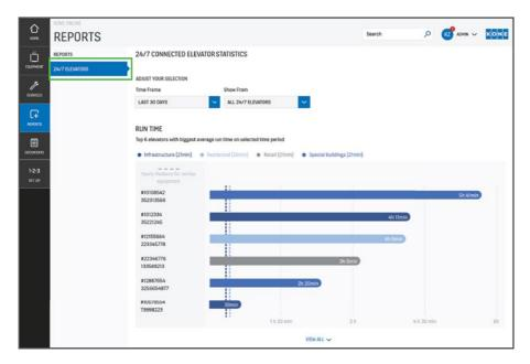
Elevators connected with KONE 24/7 Connected Services will show how long the equipment has been in operation and how many starts have occurred during the selected time period.
